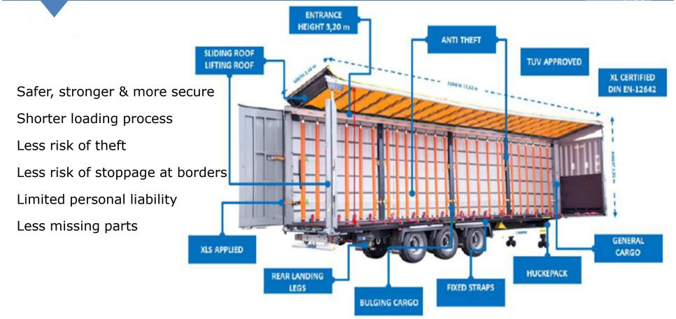
2016: 1.500 XLS trailers 2019: 3.000 XLS trailer Ewals is a pioneer when it comes to equipment development. Already in the early 90's Ewals created together with a customer and supplier the MEGA trailer. With an internal height of 2,96 m and 100 m³ capacity it has become a standard in the market. In 2011 the MEGA trailer has been further developed into the MEGA Huckepack XL version, applying the latest safety standards and intermodal capability.
